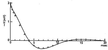
Fig. 24. Comparison of step-by-step solution and linear approximation. Eqn. (26), temperature 6°C; initial displacement of -V=2 mV. Continuous line: step-by-step solution. Circles: linear approximation with same initial displacement.
