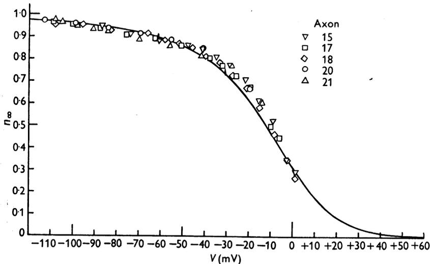
Fig. 5. Abscissa: membrane potential minus resting potential in sea water. Ordinate: experimental measurements of  $n_\infty$  calculated from the steady potassium conductance by the relation  $n_\infty = \sqrt[4]{(g_{K\infty}/\bar{g}_K)}$ , where  $\bar{g}_K$  is the 'maximum' potassium conductance. The smooth curve is drawn according to eqn. (9).
