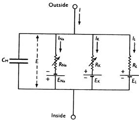
Fig. 1. Electrical circuit representing membrane.  $R_{\rm Na}=1/g_{\rm Ri}$ ;  $R_{\rm K}=1/g_{\rm K}$ ;  $R_{\rm l}=1/\bar{g}_{\rm l}$ .  $R_{\rm Na}$  and  $R_{\rm K}$  vary with time and membrane potential; the other components are constant.
