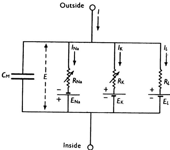
Fig. 1. Electrical circuit representing membrane.  $R_{Na} = 1/g_{Na}$ ;  $R_K = 1/g_K$ ;  $R_L = 1/\bar{g}_L$ .  $R_{Na}$  and  $R_K$  vary with time and membrane potential; the other components are constant.
