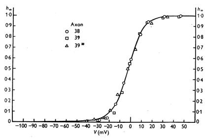
Fig. 10. Steady state relation between h and V. The smooth curve is drawn according to eqn. (25). The experimental points are those given in Table 1 of Hodgkin & Huxley (1952c). Axon 38 (5° C) as measured. Axon 39 (19° C) displaced - 1.5 mV. Axon 39\* (3° C, fibre in derelict state) displaced - 12 mV. The curve gives the fraction of the sodium-carrying system which is readily available, as a function of membrane potential, in the steady state.
