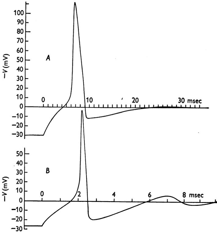
Fig. 22. Theoretical basis of anode break excitation. *A*, numerical solution of eqn. (26) for boundary condition  $-V = -30$  mV for  $t < 0$ ; temperature  $6^{\circ}$  C. *B*, anode break excitation following sudden cessation of external current which had raised the membrane potential by 26.5 mV; giant axon with long electrode at  $18.5^{\circ}$  C. Time scales differ by a factor appropriate to the temperature difference.
